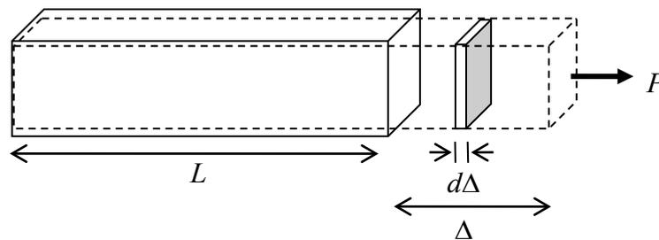
**Figure 8.2.1: a bar loaded by a force**
