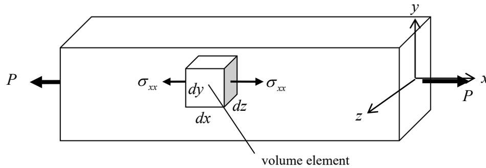
**Figure 8.2.8: a volume element under stress**
