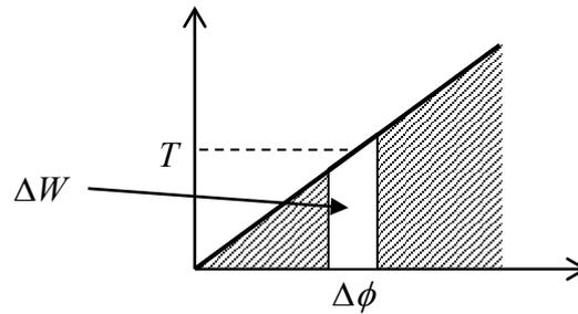
**Figure 8.2.4: torque – angle of twist plot for torsion**
