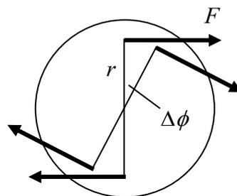
**Figure 8.2.3: torque acting on a circular bar**
