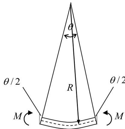
**Figure 8.2.5: beam of length  $L$  under pure bending**
