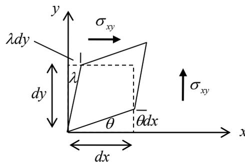
**Figure 8.2.10: a volume element under shear stress**
