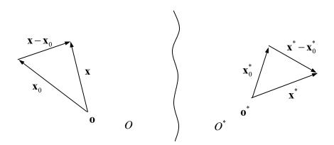
Figure 2.8.6: position vectors for two observers of the same events
