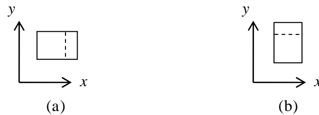
Figure 6.3.7: elements of a transversely isotropic material undergoing normal strain in the plane of isotropy
